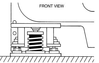
NOTE: A field supplied and installed low profile isolation is suggested to keep operation height low.
